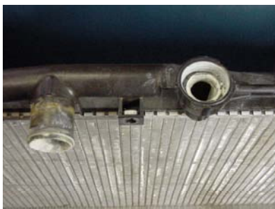
Stain on inlet and filler neck indicates the use of dirty, inhibitor depleted coolant
