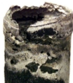
Extreme damage to inlet tubes caused by "Electrolysis and Acidic" coolant.
