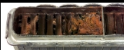
Severe damage (tubes eaten away) by corrosive and acidic coolant leading to failure at the tube to header joint.
