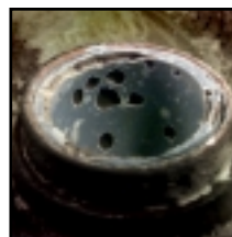
Extreme damage to inlet tubes caused by "Electrolysis and Acidic" coolant.
